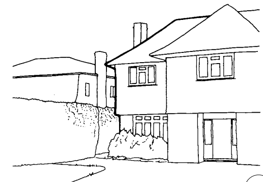
Figure 4.8: Negative example: Houses merge with one another and the hedge alone does not provide an appropriate landscape screen or adequate gap.
