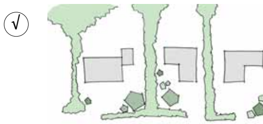
Figure 4.11: Detached housing can sit comfortably in its site with space for planting and sufficient gaps between buildings.
