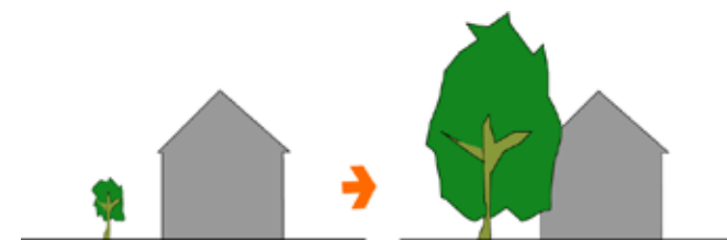
Figure 7.2: Sketch illustrating the principle of buffer zones around planting. Distance between tree, hedge or shrub planting and any foundations to ensure that the plant can grow and develop healthily. Distances depend on species, anticipated canopy size and root protection area.
